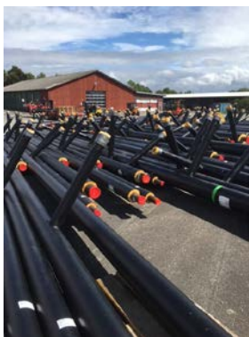
Fig. 8 and 9 - Standpipes made indoor. In the indoor factory straight pipelines are manufactured with standpipes, designed so they match the exact position of the solar panels.
