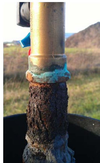
Fig. 3 - Released copper ions from brass valve, causing corrosion of the steel pipe. The damage is on the return pipe. No damage on the flow pipe.
