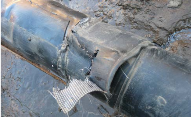
Fig. 4 - Shrink wrap peeled off due to the large number of movements.
