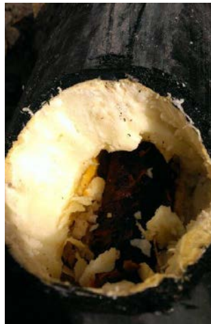
Fig. 2 - Moisture spread, stemming from a casing joint, damaged by large movements.
