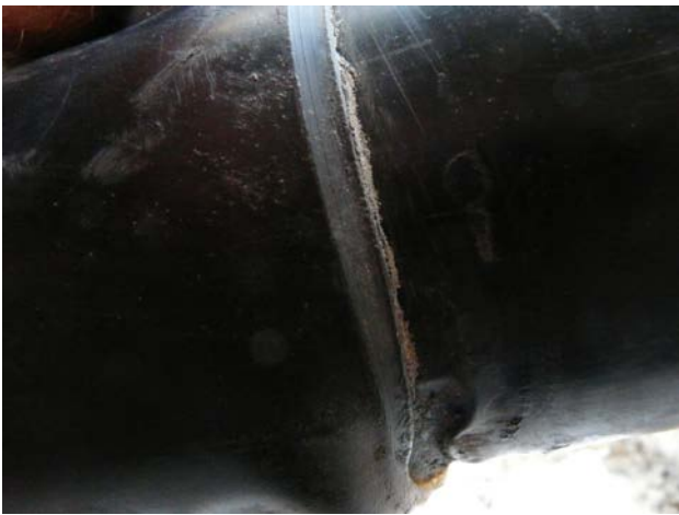
Fig. 5 - Dislocated casing joint due to the large number of movements
