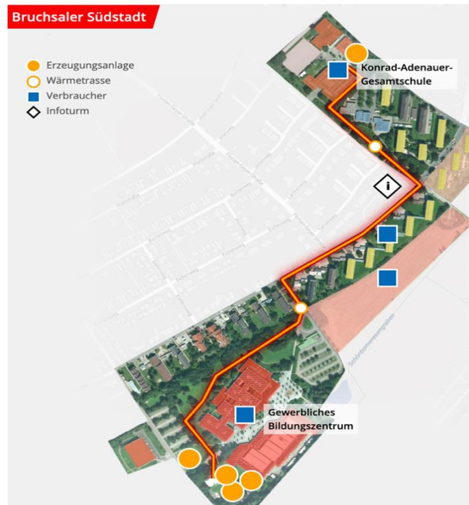
Figure 10. Map of the planning of the district heating network in Südstadt, Bruchsal (Stadtwerke Bruchsal, 2021)
